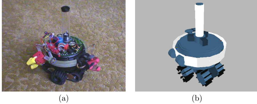
Figure 2: The s-bot . (a) The prototype of the s-bot . (b) A graphical representation of the simulation model which closely reproduces the mechanical structure of the s-bot , as required by our experiments.
