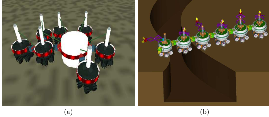
Fig. 1. Graphic visualisation of how the rigid gripper can be used to connect in a secure way s-bots among themselves so to form a swarm-bot for (a) retrieving heavy objects or (b) passing over holes.
