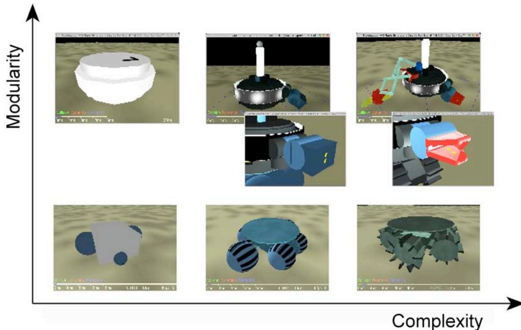
Figure 7: The simulation of the s-bot hardware is structured into various modules, each of them modeled at several levels of complexity. These features allow a very flexible simulation, adjusting in an optimal way the simulation complexity to the experiments.
