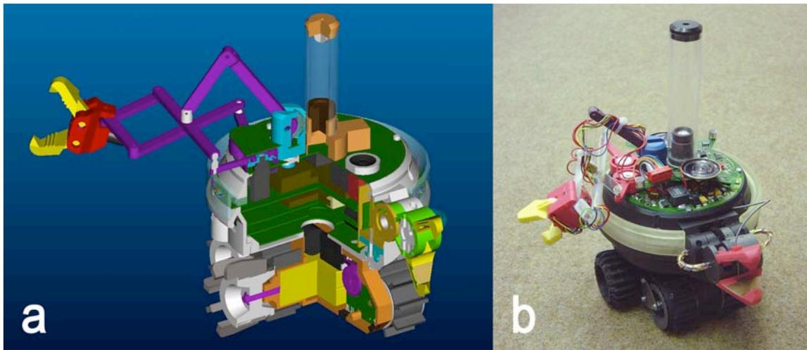
Figure 3: Detailed design and final implementation of an s-bot. The diameter of the robot is 120 mm.
