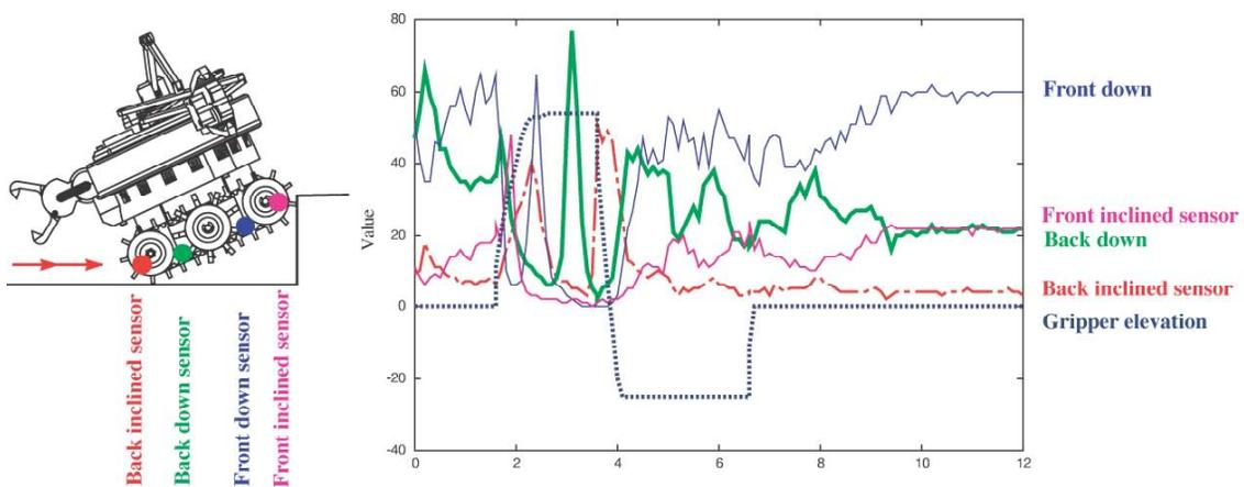
Figure 6: Activation of ground distance sensors and actuation of the gripper elevation for the first of the two s-bots in the step-passing problem illustrated in figure 5.
