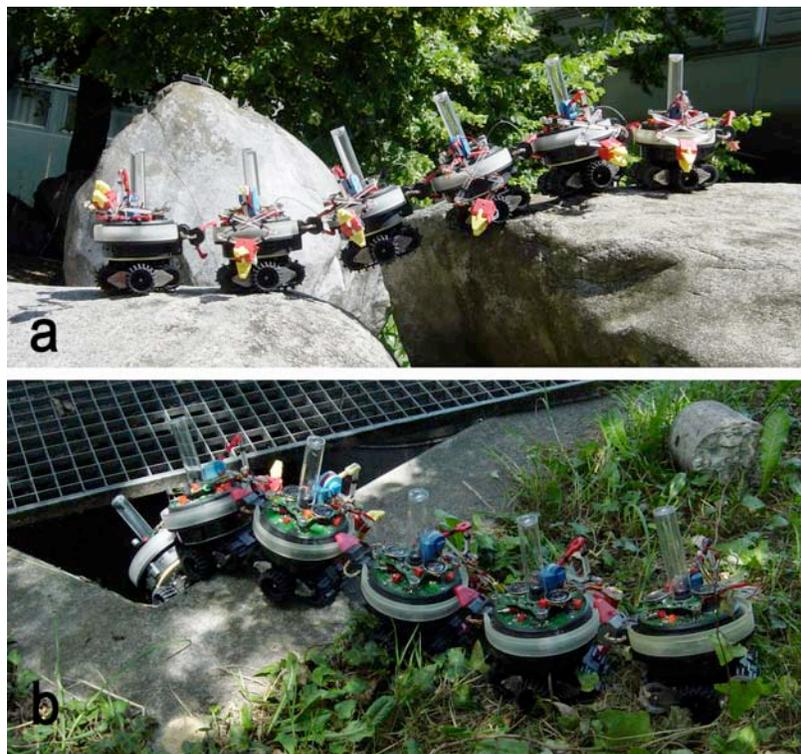
Figure 1: Swarm-bots in situations of extreme all-terrain navigation where chain formation is exploited for (a) passing a gap and (b) going through a narrow passage.
