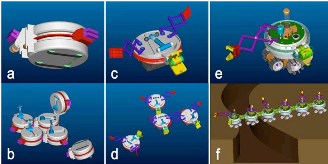
Figure 2: Evolution of the swarm-bot hardware design. (a-b): Results of the first brainstorming. (c-d): Introduction of flexible links and better mobility. (e-f): Choice of gripper-based connections and design finalization.
