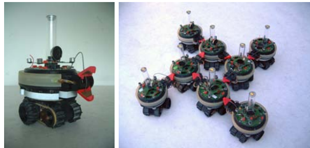
Fig. 1. Left: An s-bot . Right: A “star-shaped” swarm-bot composed of 8 s-bots .
