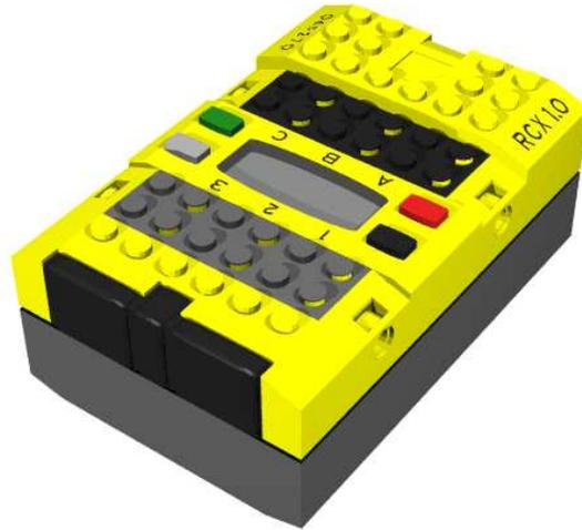
Figure 3.2: A picture of the Brick included in each Lego Mindstorm™ box. The infrared transmitter is in the front. On the top there are an LCD display, four keys, three slots for sensors (the front grey stripe) and three slots for actuators (the back black stripe).
