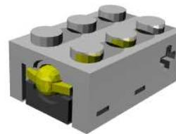
(d) Touch sensor. It is a simple switch that turns on when the front button is pressed.
