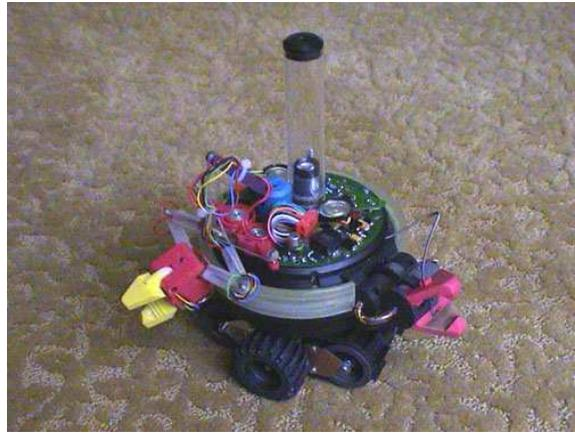
Figure 3.2: One of the two first *s-bot* prototypes.
