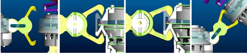
Figure 2.4: *S-bot* gripper. The mechanism by which one *s-bot* connects to another.
