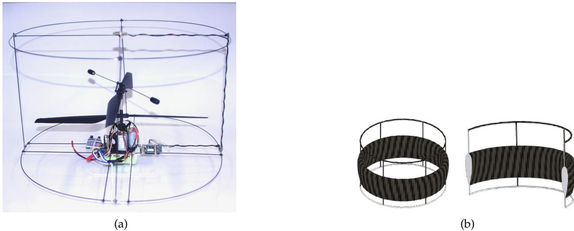
Figure 1.3: Eyebot design: (a) the eyebot prototype hovering platform and (b) the designed aerodynamic ducts.
