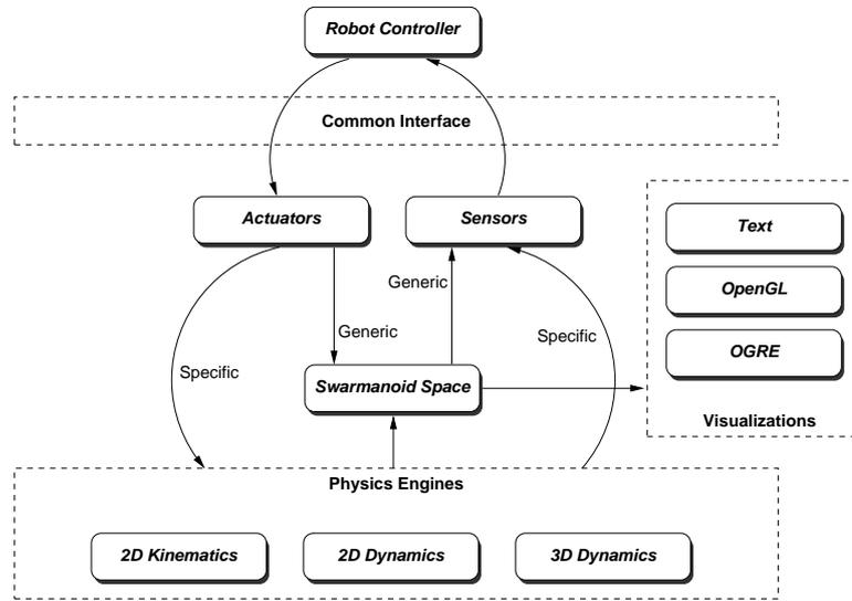
Figure 3.1: Overall architecture of the simulator.
