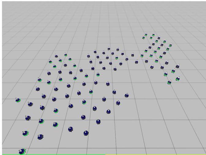
Figure 3.7: A condition of unsuccessful flocking behavior. The swarm after while splits in different groups. The aligning robots are able effectively flock, whereas the non-aligning ones are unable to keep the pace.
