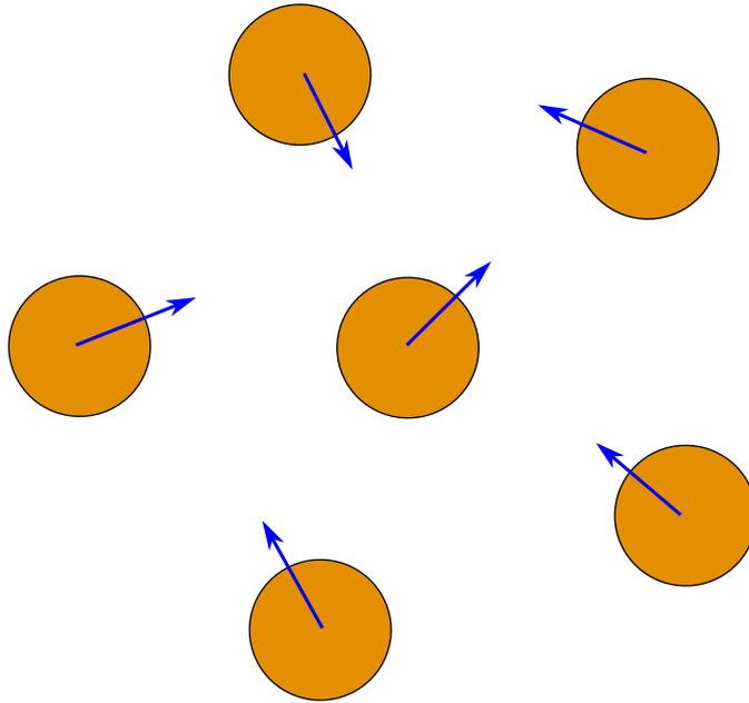
Figure 2.1: In the artificial physics framework used in this work, robots exert forces on each other and move according to the resulting forces acting on them, represented here by the blue arrows.
