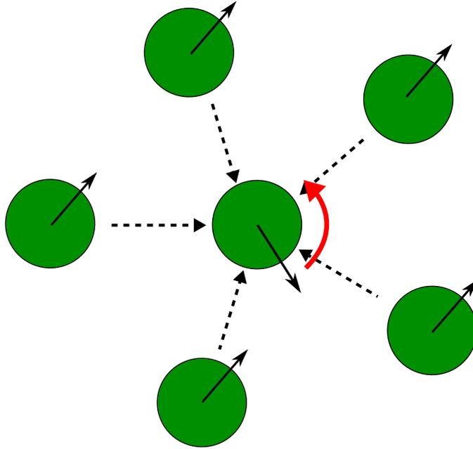
Figure 2.5: Alignment control behavior representation.
