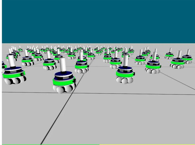
Figure 3.2: A swarm of simulated Foot-bots in ARGoS.
