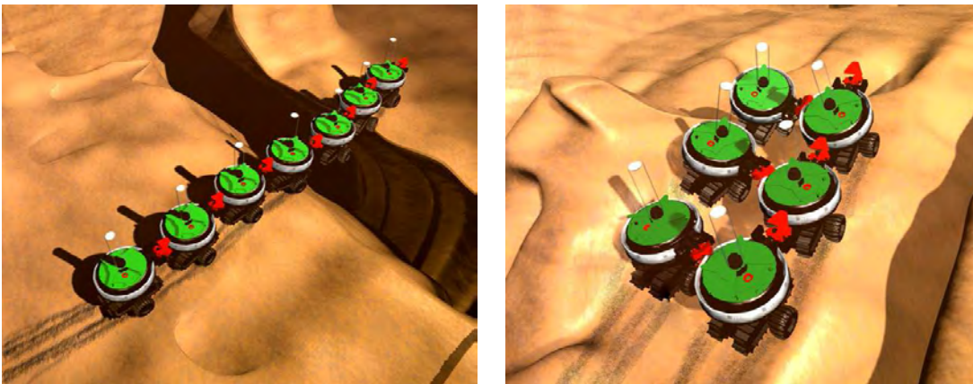
Figure 1.1: Two examples of robotic entities self-assembled into morphologies appropriate for the task. Left: A connected robotic entity crosses a trough. A line formation is well-suited to this task, since it allows the entity to stretch further and requires only a minimum number of robots to be suspended over the trough at any one time. Right: A more dense structure provides greater stability for rough terrain navigation.
