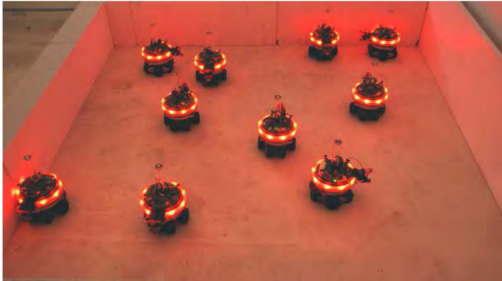
Figure 5.7: A photo of synchronized robots flashing at the same time.
