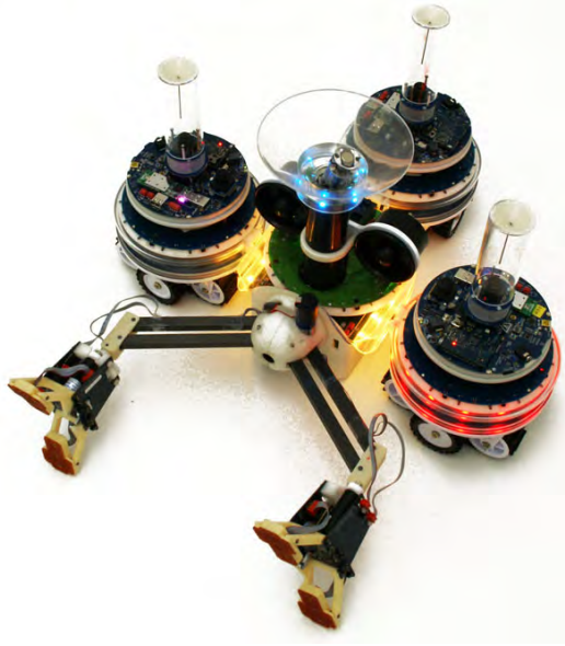
Figure 5.1: Picture of robot setup: three mobile robots are attached to an irregularly shaped object, another robot, that can only be grasped only in certain regions.
