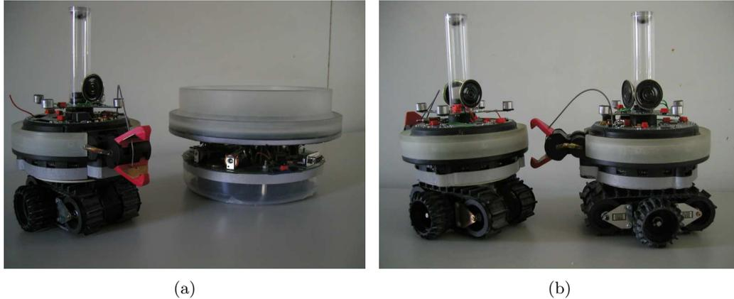
Figure 10.3.: A single s-bot self-assembling with (a) an object, called the prey, and with (b) a teammate.
