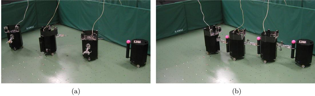
Figure 12.7.: A group of four robots self-assembling: (a) initial configuration and (b) final configuration reached after 475 s. In this experiment, the robot on the right acts as a seed to the process. Once a robot has established a connection, a visual mark is manually attached to the coupling cylinder at its back.
