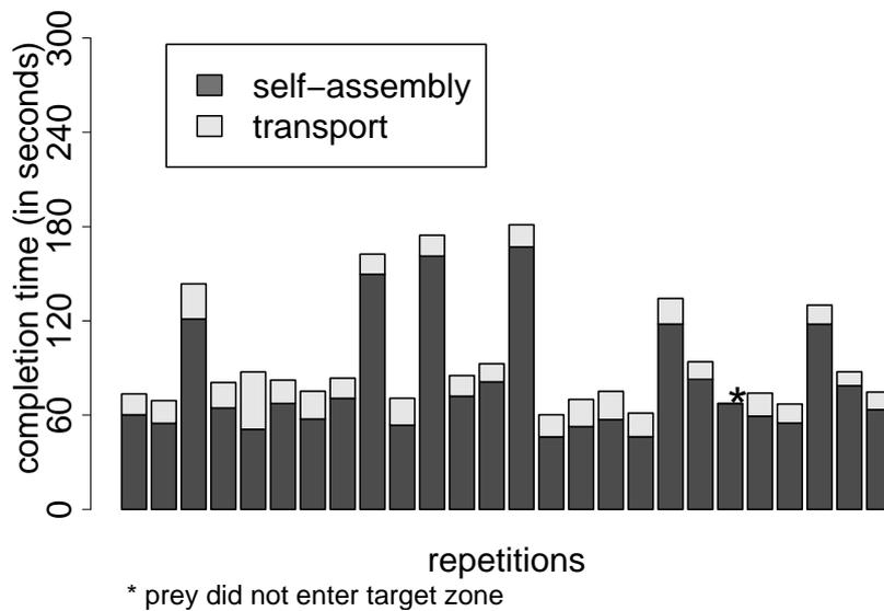
Figure 16.5.: Time necessary for a group of six s-bots to self-assemble and transport the prey inside the target zone (only repetitions in which all s-bots assembled).
