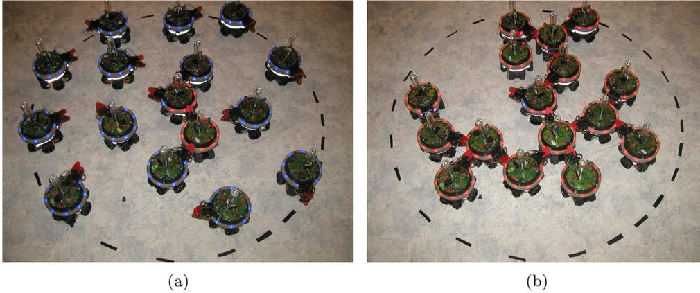
Figure 10.10.: Self-assembly of 16 physical s-bots put in a circle of radius 50 cm.
