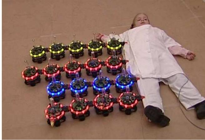
Figure 17.1.: Rescue scenario: 19 s-bots organized into four distinct pulling chains transporting a child. One s-bot was manually removed during experimentation as its connection mechanism broke. This work was accomplished in collaboration with I. Aloisio, M. Bonani, F. Mondada, A. Guignard, and D. Floreano.
