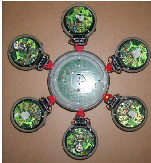
Figure 15.4.: Experimental setup. An object has to be transported towards a target (on the bottom; not shown). Six s-bot are manually attached to the object. While some s-bots are fully operational, others are not capable of perceiving the target.
