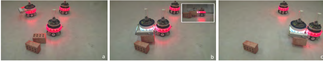
Figure 3.10: MNS robot borrowing physical capabilities from a peer robot. (a) Two foot-bots and a manipulator foot-bot are deployed on an object transport task. (b) A foot-bot has detected a suitable brick to be transported and extends its morphology to acquire new physical capabilities available exclusively to the manipulator foot-bot. (c) The new composite MNS robot is able to successfully transport the brick.
