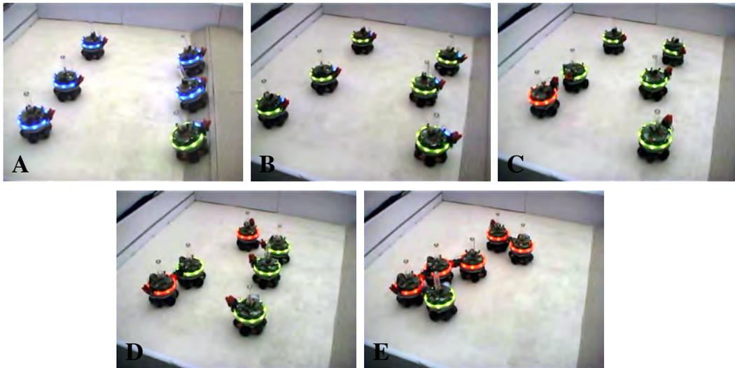
Figure 5.14: Scalability experiment in the difficult hill environment: 6 s-bots using the *basic self-assembly response* strategy self-assemble into two groups, both of which successfully cross the hill.
