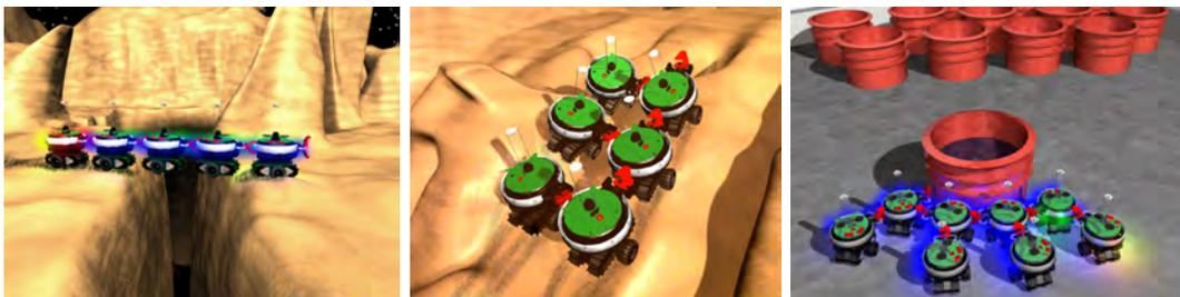
Figure 8.1: Three examples of robotic entities self-assembled into morphologies appropriate for the task. Left: A connected robotic entity crosses a trough. A line formation is well-suited to this task, since it allows the entity to stretch further and minimises the number of robots suspended over the trough. Centre: A more dense structure provides greater stability for rough terrain navigation. Right: A pushing morphology appropriate for moving heavy objects.
