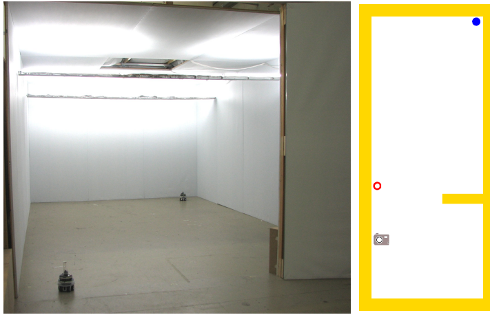
Figure 6.4: Setup of the validation experiments of Section 6.2. The picture on the left shows the real arena in which the experiments were conducted. The target locations the robots must visit are marked by dedicated robots. The diagram on the right depicts the equivalent simulated arena. The empty and filled circles represent the target positions, and the camera marks the location in which the picture on the left was taken.
