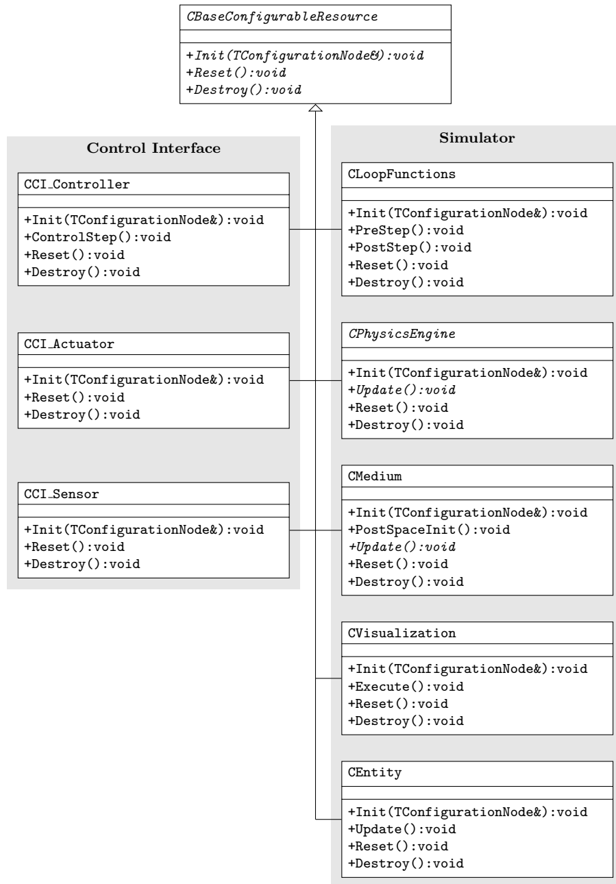
Figure 4.2: A UML class diagram of the basic plug-in hierarchy in ARGoS.
