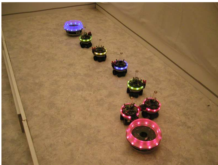
Figure 5.8: The scenario solved. Six s-bots are involved in the experiments. Four of them are aggregated into a robot chain, and two are assembled to the prey (red object). The blue object represents the nest, which is also the target location of the collective transport.
