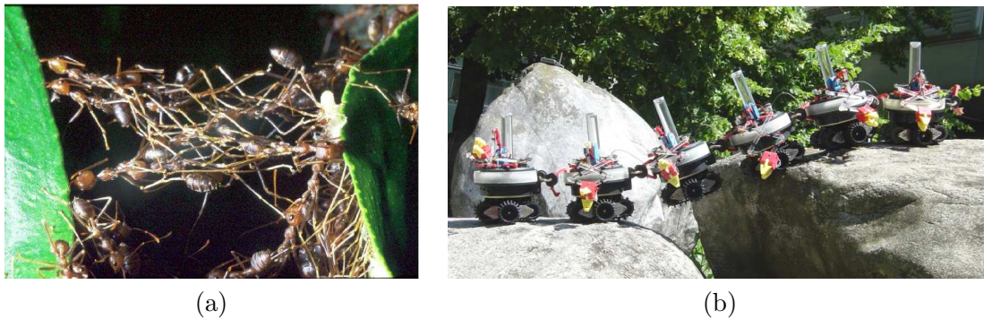
Figure 10.1: Examples of self-assembly observed in ants and robots. (a) Ants of the species Ecophilla longinoda forming a chain (This image has been kindly provided by Dr. Arnaud Lioni). (b) A demonstrative image of a swarm-bot structured in a chain while passing over a trough.
