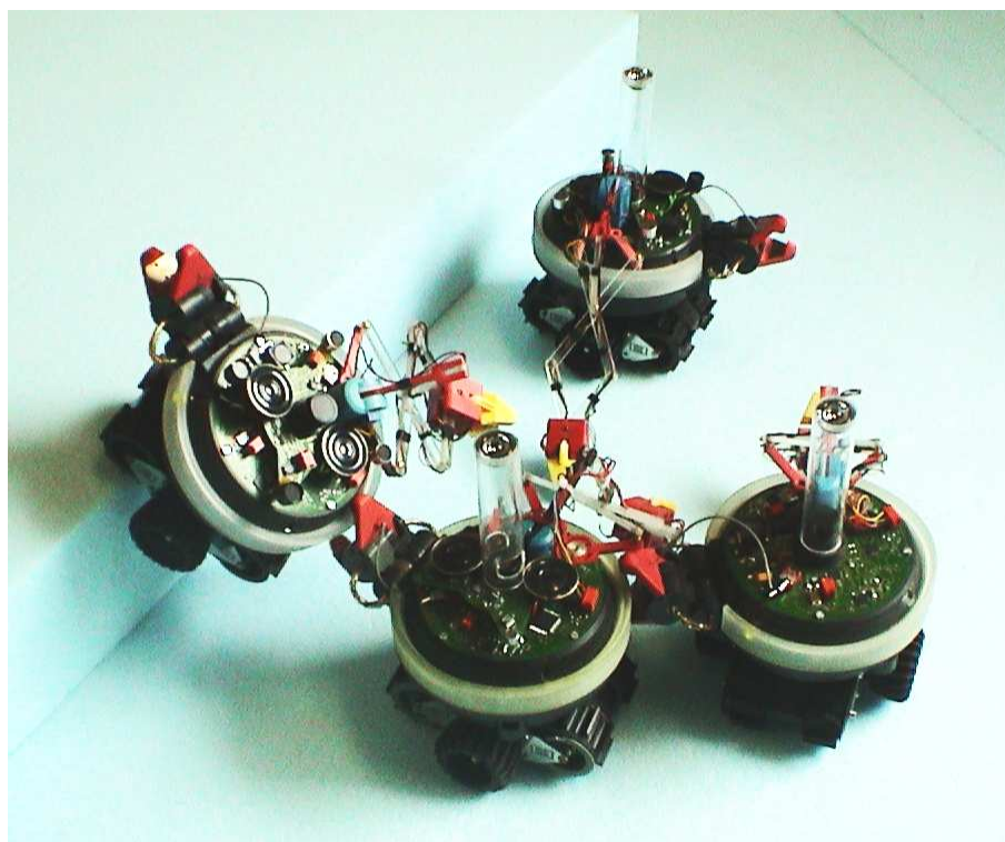
Figure 5.2: Four s-bots connected in different ways to form a swarm-bot . The elevation of the rigid gripper allows to lift an s-bot , opening to the possibility of climbing steps or other obstacles. All s-bots shown are equipped with a flexible arm, characterised by three degree of freedom and a gripper mounted as end effector.
