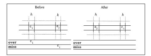
Figure 8. Swapping two elements (a class and a movable gene).
