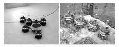
Fig. 2. Left: 6 s-bots, of which 4 in swarm-bot formation, collaborate to transport a heavy object. Right: A 4 s-bots linear swarm-bot moves on rough terrain.
