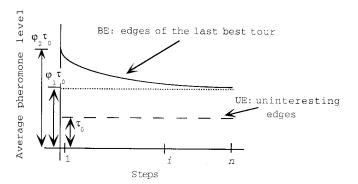
Fig. 6. Change in average pheromone level during an algorithm iteration for edges in the BE family. The average pheromone level on edges in BE starts at  $\varphi_2\tau_0$  and decreases each time an ant visits an edge in BE. After one algorithm iteration, each edge in BE has been visited on average  $m\cdot q_0$  times, and the final value of the pheromone level is  $\varphi_1\tau_0$ .
