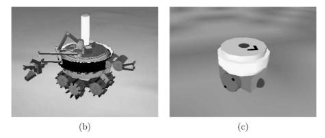
*Figure 1.* The *s-bot.* (a) The first prototype of the *s-bot* (the diameter of the main body is 116 mm). (b) A graphical representation of the detailed simulation model which closely reproduces the mechanical structure of the *s-bot.* (c) A graphical representation of the simplified model, in which the details of the *s-bot* unnecessary for our experiments are omitted. Both the detailed and the simple models are implemented using physics-based software libraries.
