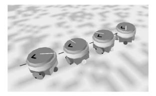
*Figure 7.* Four physically linked *s-bots* forming a linear structure. The line between two *s-bots* represents the physical link between them. The white line above each *s-bot* indicates the direction and intensity of the traction.
