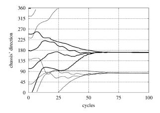
*Figure 10.* The graph shows the direction of the chassis of the four *s-bots* during 150 simulation cycles, starting with two different initial random orientations (continuous and dotted lines, respectively).
