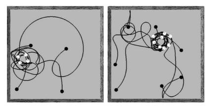
*Figure 4.* Aggregation behavior. (a) The aggregation of 4 *s*-*bots* usually produces groups moving in circles. (b) When the group is bigger, the movement is more disordered and the *s*-*bots* continuously change their relative positions.
