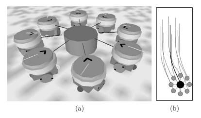
*Figure 14.* (a) Eight *s*-*bots* connected to an object through rigid links. (b) Traces left by the *s*-*bots* (thin lines) and the object (thick line) during 150 simulation cycles. The gray and black circles represent the initial positions of the *s*-*bots* and of the object.
