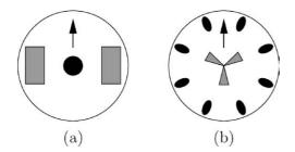
*Figure 2.* A schematic *s-bot* seen from the top. The arrows show the front direction. (a) Actuators: the two gray rectangles indicate the motorized wheels. The black circle indicates the speaker, which continuously emits a sound. (b) Sensors: 8 proximity sensors (black ellipses) and three directional microphones (gray triangles).
