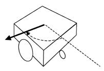
*Figure 8.* Traction force detected by the *s*-*bots*' traction sensor. The large and small circles respectively represent the right active wheel and front passive wheel. The dashed line and the full arrow respectively indicate the chassis' orientation and the direction and intensity of the traction. The dashed arrow indicates the angle between the chassis' orientation and the traction.
