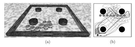
*Figure 13.* Eight *s-bots* assembled into a snake formation displaying collective obstacle avoidance. (a) The parallelepipeds and the large cylinders represent walls and obstacles, respectively. (b) The small gray circles represent the initial position and shape of the *swarm-bot*. The square and the large full circles represent the walls and the obstacles. The lines show the trajectory of the *s-bots* during 600 simulation cycles.
