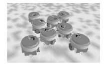
Figure 11. Eight s-bots connected by rigid links into a star formation.
