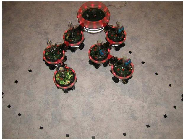
**Figure 11.** (a) Above: Self-assembly of six *s-bots* with an *s-toy* (34 repetitions). (b) Below: Self-assembly on different types of terrain: percentage of successful connections (from the left box to the right box: 160, 204, 40, 120, 40, and 120 observations). The percentage of connected *s-bots* is 91% for the most challenging setup (6 *s-bots*, very rough terrain).
