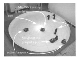
**Fig. 2.** Snapshot of an experiment. Four *MindS-bots* are looking for three prey. The nest is indicated by a light in the centre. One *MindS-bot* is resting in the nest, two are exploring the environment, and the fourth is retrieving a prey to the nest.
