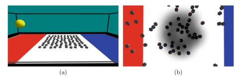
Fig. 1. View of the environment and Kilobot swarm implemented with the ARGoS3 simulator (a) and of the SHCS during a simulated experiment (b). The shaded area shows the communication range of the SHCS considered as a whole. SHCS robots show their LED in green (seed robot) or white (remaining SHCS robots); robots showing blue and red LEDs are SO robots, with the color representing their current opinion. (Color figure online)
