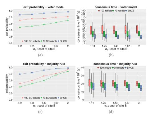
**Fig. 2.** Simulation results with SHCS, 100 SO robots, and 70 SO robots for varying  $\sigma_B$ : exit probability (a) and consensus time (b) for the voter model; exit probability (c) and consensus time (d) for the majority rule. Results obtained running 1000 simulations for each tested condition.
