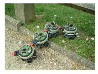
**Fig. 1** A *swarm-bot* moving in an outdoor environment. The traction system of each *s-bot* is composed of both tracks and wheels. On top of it, a rotating turret is mounted, which holds many sensory systems and the rigid gripper for physical connections
