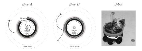
**Fig. 1.** Depiction of the task and picture of a *s-bot* close to a 1 Euro coin. The *dark* zone is the area within the dotted circles. The target area, centred on the light, is indicated by the dashed circle. The continuous arrows are examples of good navigational strategies.
