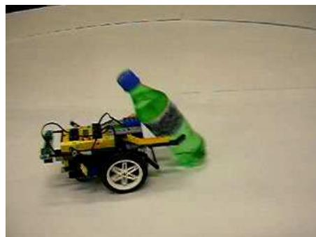
(b) The friction of the prey with the ground is too high for the gripper.
