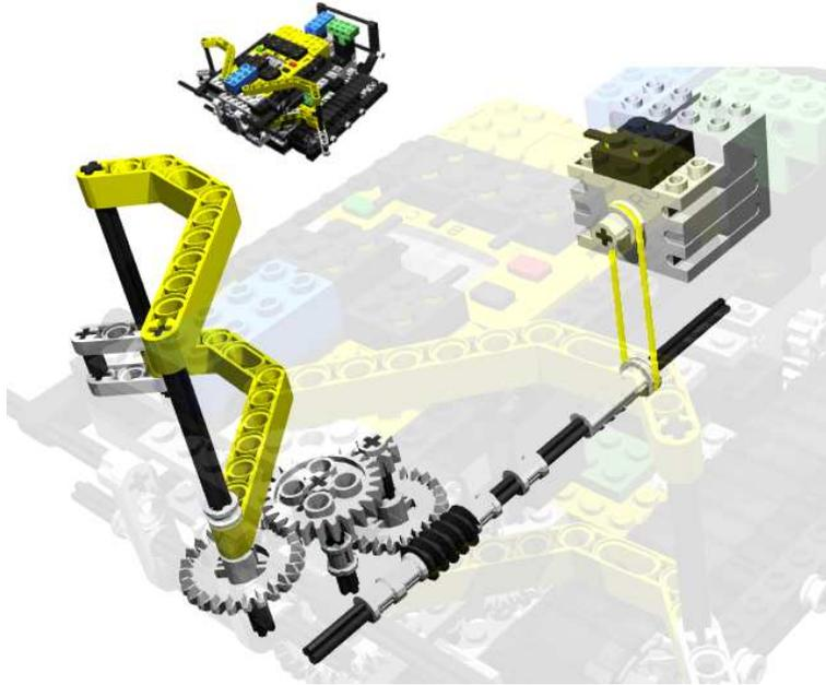
Figure 3.8: Details of the gripper. The series of gears create a reduction which is strong enough to block the gripper without short-circuiting the motor. The parts of the robots that are not of interest are transparent. On the top, a small picture shows the perspective of the *MindS-bot*.
