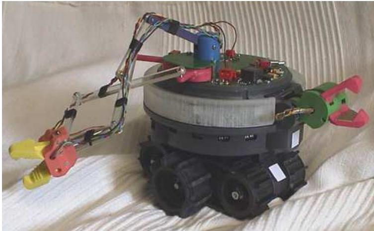
Figure 1.3: The hardware prototype of an *s-bot*.
