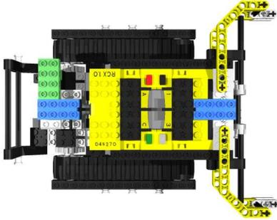
(a) Top view of a *MindS-bot*. The blue bricks are light sensors. The gripper arms are half opened to have an idea of the grasping area. The front bumper takes less space on the horizontal axis than the back one in order to permit an easier grasping of prey.
