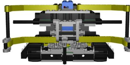
(b) Front view of a *MindS-bot*. The front light sensor is on the top. The whiskers of the bumper occupy nearly all the area to detect possible collisions more easily.
