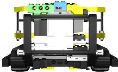
(c) Back view of a *MindS-bot*. This part is mainly covered by the back bumper for collision detection when moving backward. Behind it, there are the three motors for the tracks and the gripper. On the top there is a light sensor.
