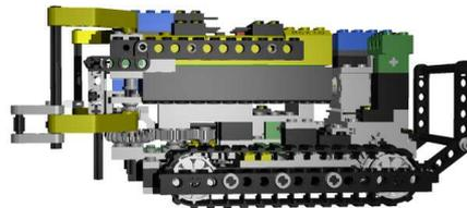
(d) Side view of a *MindS-bot*. Tracks do not occupy vertical space that can be used by the gripper's arms when it is open.
