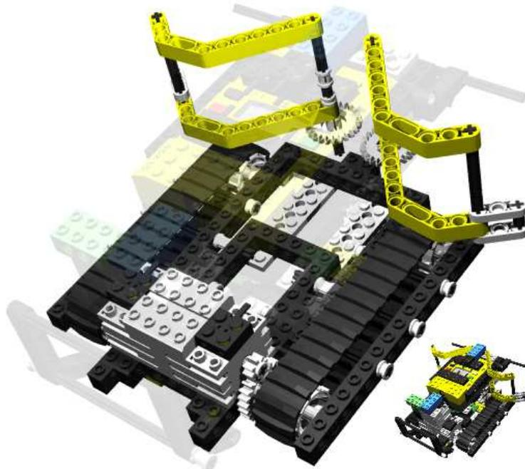
Figure 3.7: Details of the traction system. The gripper's arms can be placed over the tracks when the gripper is open. A small reduction in the transmission between the motors and the tracks allows for a stronger traction at the cost of a slower speed. The parts of the robots that are not of interest are transparent. On the bottom right corner, a small picture shows the perspective of the *MindS-bot*.
