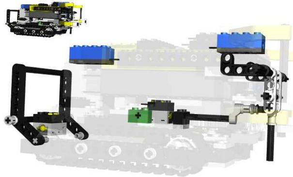
Figure 3.10: Details of the sensors. Light sensors are on the top to reduce problems with the shadows of other *MindS-bots*. The back touch sensor is pressed when the back lever is pushed against the *MindS-bot*. When the front whisker is pressed, an axle connected to it pushes the button of the touch sensor that is placed under the Brick. The parts of the robots that are not of interest are transparent. On the top left corner, a small picture shows the perspective of the *MindS-bot*.
