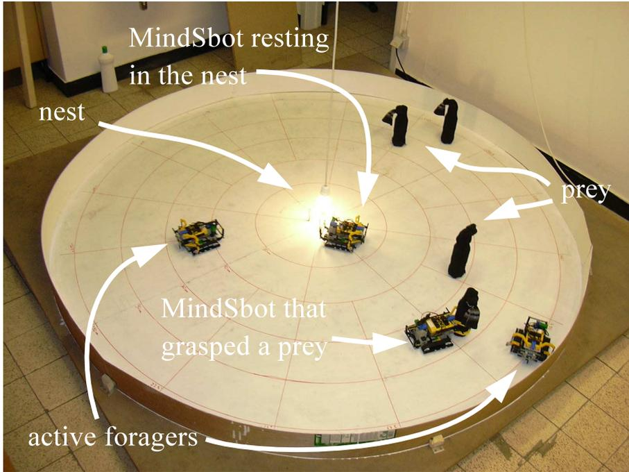
Figure 5.3: Snapshot of an experiment. Four *MindS-bots* are looking for three prey. The nest is indicated by a light in the centre. One *MindS-bot* is resting in the nest and is therefore inactive. Two others are exploring the environment. One found a prey. It grasped it and is searching for the nest to retrieve it.
