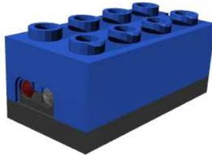
(c) Light sensor. On the front there are a red LED and the actual sensor.
