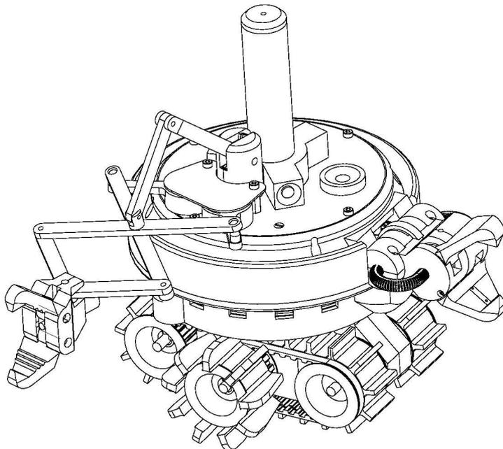
Figure 1.2: The design of an *s-bot*.
